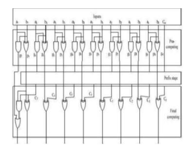
In pre computation stage, propagates and generates are Computed In the prefix stage, the black cell (BC) and gray cell (GC) generates only the building prefix structures. Final computation, the sum and carryout are the final output. Black Cell and Gray Cell
